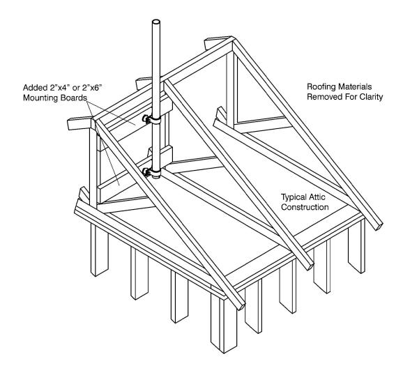
Mounting Through a Roof or Roof Overhang
