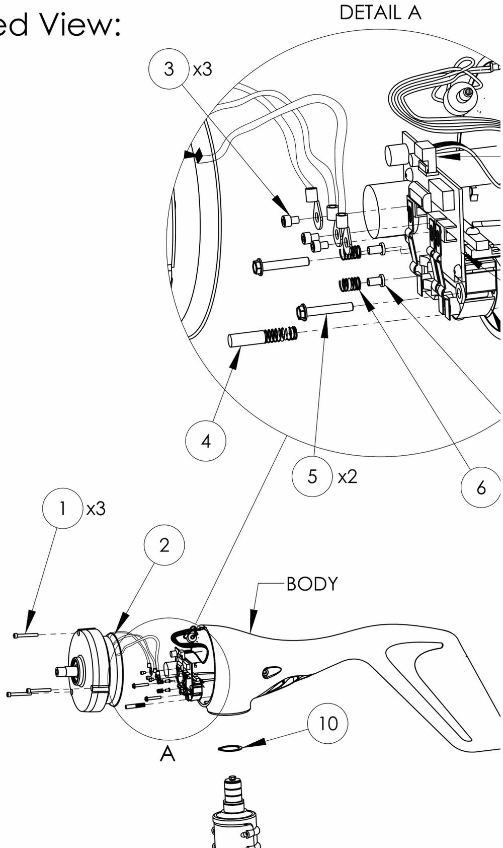
1. Disconnect the wires and remove the turbine from the mount as per the AIR X or AIR BREEZE Owner's Manual, Section 6. Remove the nose cone, then the blade assembly with a  $\frac{5}{16}$ " hex key.
